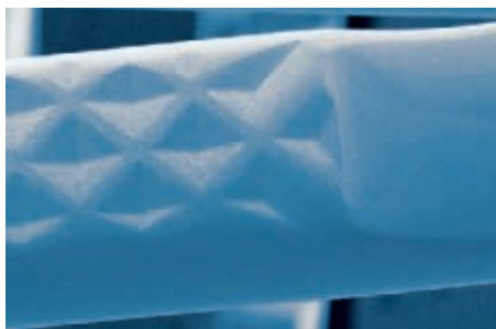
REM image atraumatic blade profile of a YASARGIL Clip from Aesculap; the deep, symmetrical, pyramidal stamping of both blades doubles the contact surface area and counteracts the slip effect.
