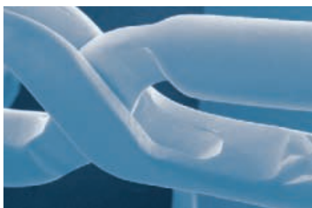
REM image patented box lock of a YASARGIL Clip from Aesculap; the flat design with a broad contact surface ensures smooth opening and closing, stability and safety.
