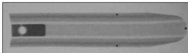
Placement of the stainless steel pins on the Soft Tissue Retractor
